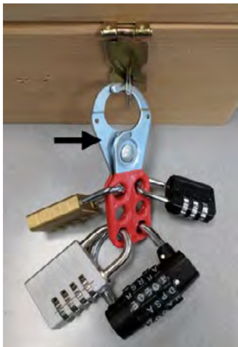
Figure 1. A hasp, (indicated with a black arrow), holding a variety of locks on an escape box.
